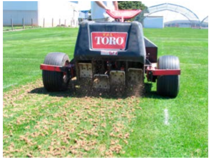
Figure 3. Hollow-tine aerification temporarily disrupts the soil surface, but it is one of the best things you can do for the health and performance of your field.
